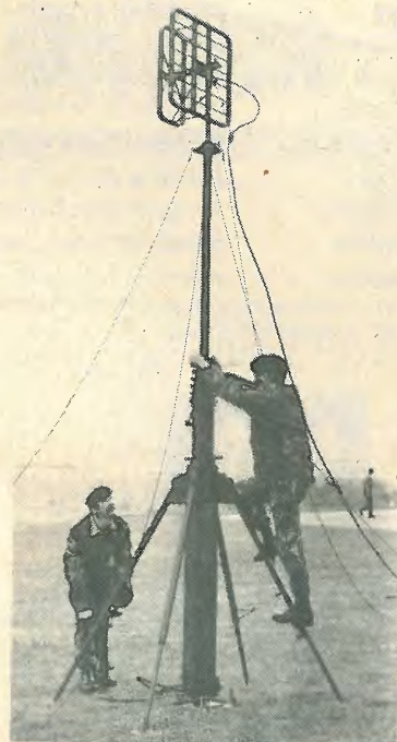
SCAM Telescopic air-operated 12-metre mast kit shown in radio relay role for field or vehicle mounting 9-, 12-, 15- and 21-metre versions available.
